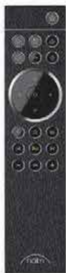
LEFT: Illuminated keys on Naim's RF 'Zigbee' remote allow full access to its menu and features even in low-light conditions
