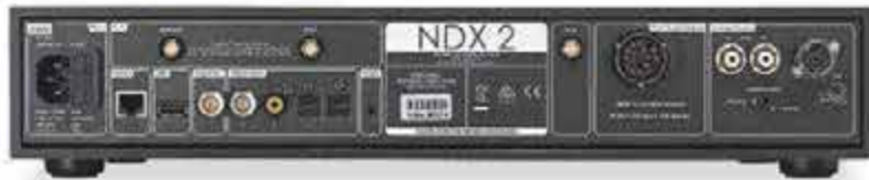
ABOVE: Two Toslink optical and coaxial digital ins (one on BNC) are joined by USB-Type A and wired/wireless Ethernet for network audio. Outputs are on RCAs and a 5-pin DIN. Note the large connector to accommodate a DR-series PSU upgrade
