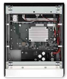
ABOVE: The 12V/4A external supply is routed through to additional regulation [bottom] while the mainboard processor is screened and cooled under a heatsink
