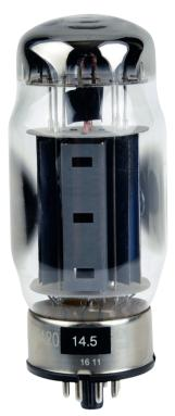
In order to preserve the typical spectrum of an SE amp, the KT120 is run in pure triode mode in the Octave V16.
