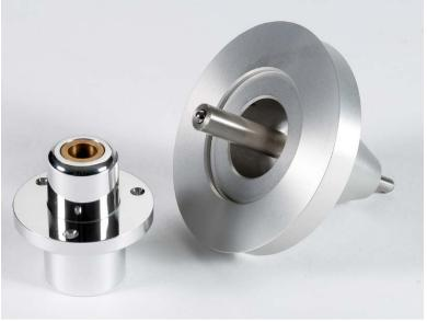
The case of the MC-pickup consists of a solid aluminum block. The needle carrier is made of hard sapphire. The diamond has a sophisticated "Shibata"-cut.
